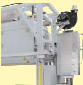
Catalytic post combustion integrated on the furnace housing to save space
