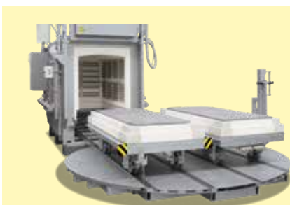
Turntable to exchange bogies in front of the furnace
