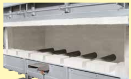
Indirect gas firing with radiation tubes
