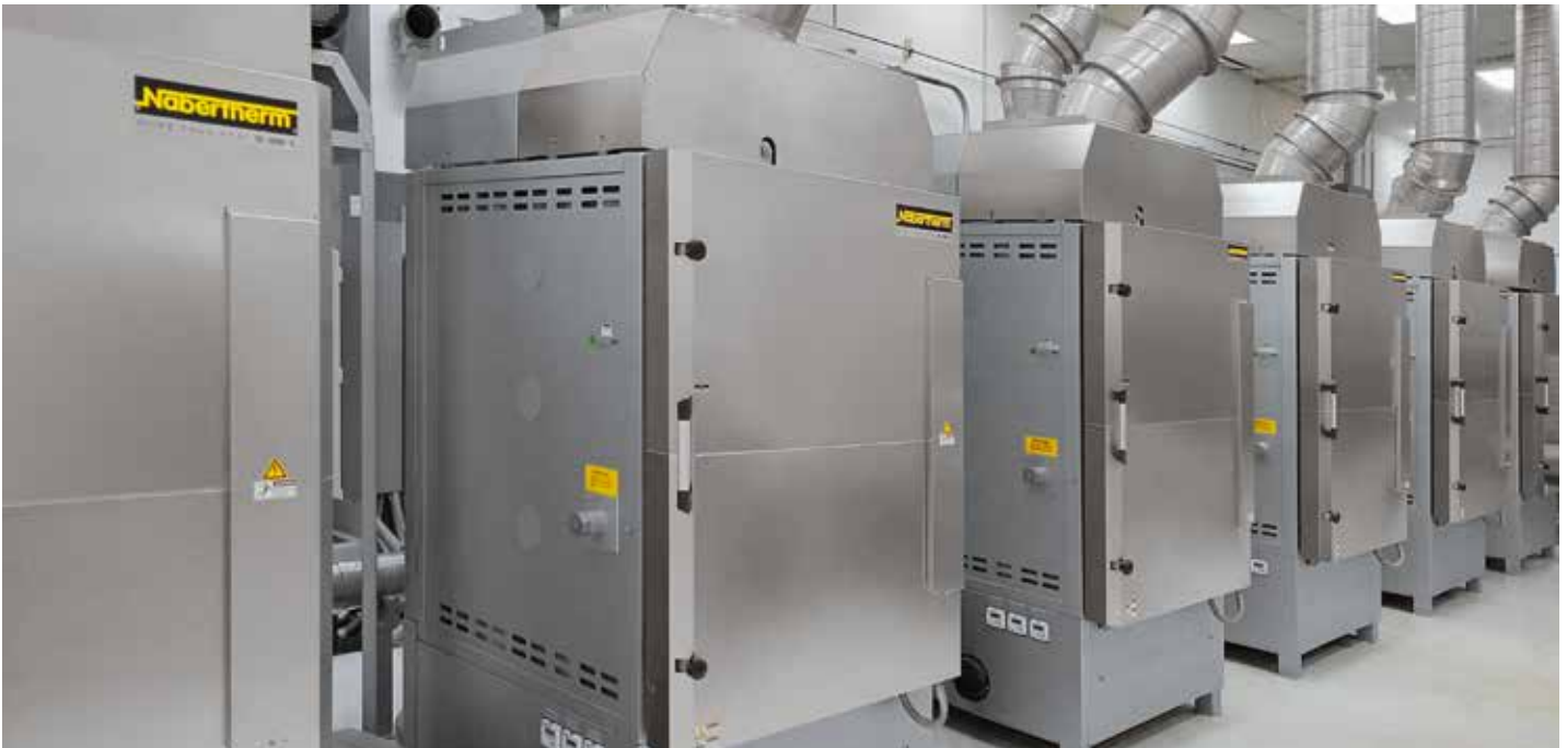
Production line consisting of combi chamber furnaces N 650 DB200 with catalytic post combustion for alternating operation
