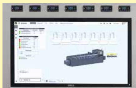
Display of all settable values via NCC (e.g. temperature monitoring for heating zones, flow rates of gassing)
