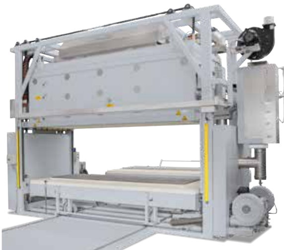
Top hat furnace H 3000 DB200-3 with interchangeable table system for two tables and catalytic post combustion system KNV 320 installed on the housing
