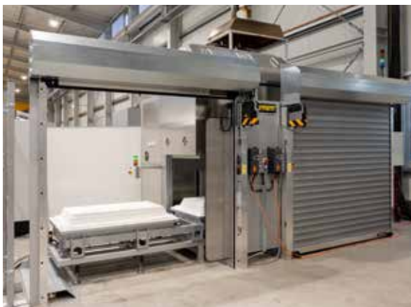
High-temperature top hat furnace HT 400/17 LT DB200-4 with roller doors for automatic table exchange
