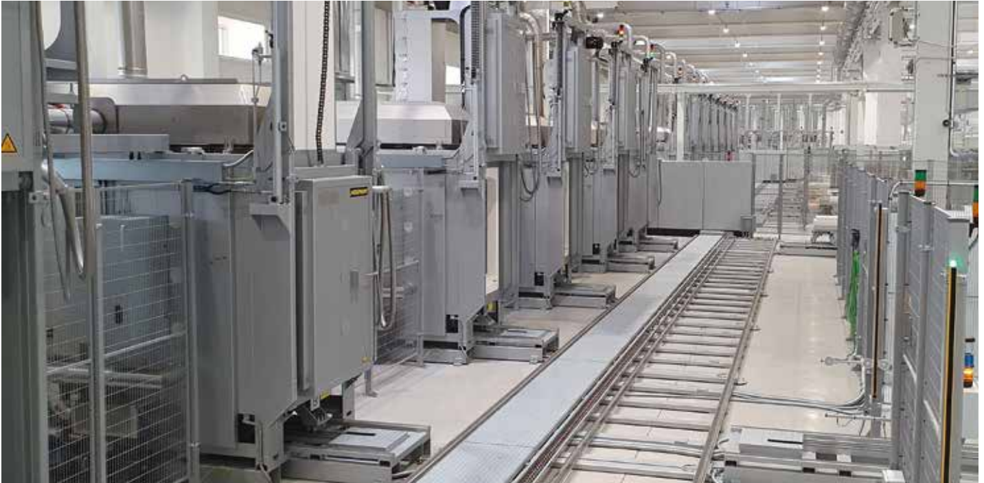
Furnace system with six combi bogie hearth furnaces W 2254/14 DB200-3 with catalytic post combustion for alternating operation, lift door and transfer system with loading/unloading station for automatic operation
