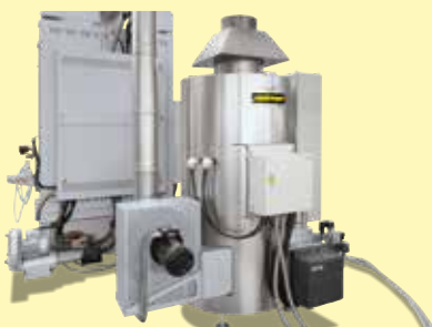
Catalytic or thermal post combustion as additional equipment available (picture shows thermal post combustion)
