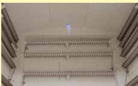
Furnace chamber N 300 BO with gas-operated pilot flame and electric furnace heating
