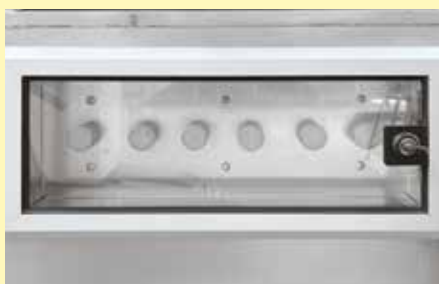
Adjustable gas injection for clean, dry air (CDA). Can be locked to increase process safety
