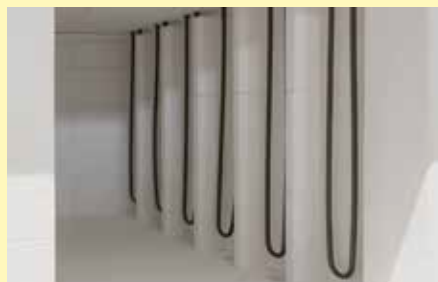
Protection of heating elements against mechanical damage during loading and unloading as additional equipment
