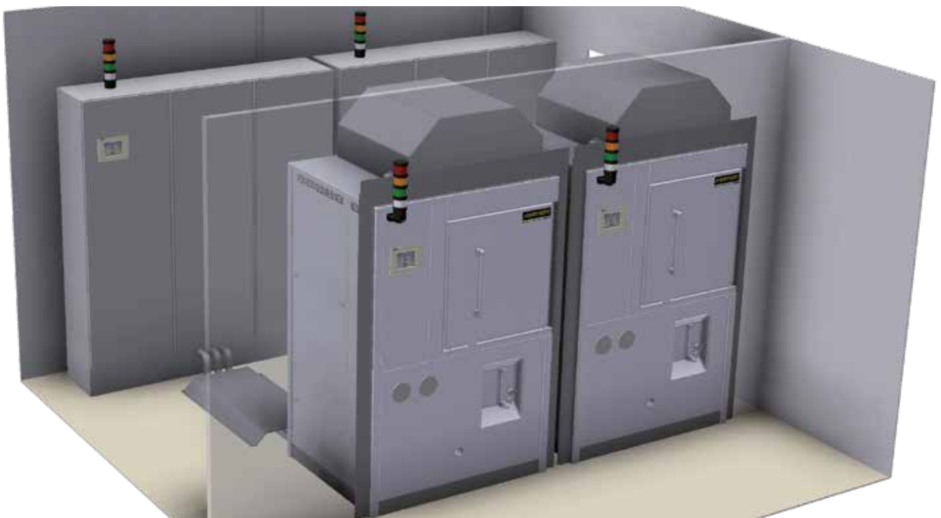
High-temperature furnace with loading from the clean room; switchgear and furnace installed in grey room
