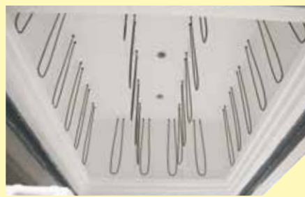
Heat from all sides and between the stack to optimize temperature uniformity
