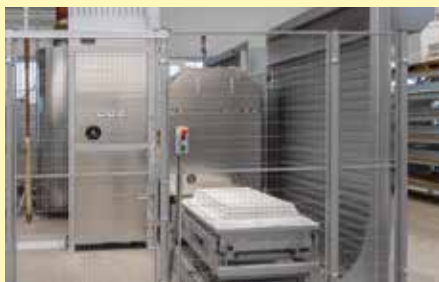
Safety zone protected with roller doors and safety barrier
