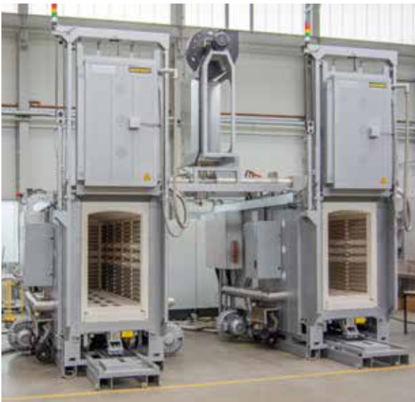
Two combi bogie hearth furnaces W 2254/14 DB200-4 with catalytic post combustion for alternating operation
