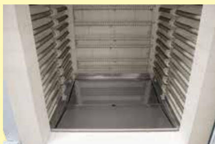
Drain pan in floor
