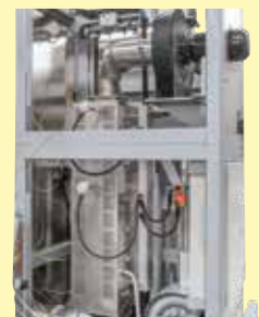
Catalytic post combustion to clean the exhaust air as additional equipment
