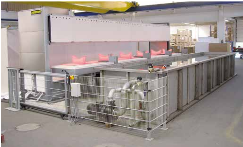
Tempering plant with top hat furnace H 4263/12S and water bath
