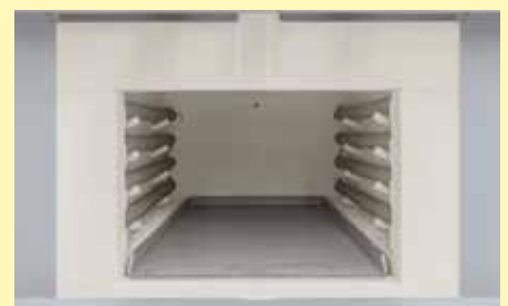
Deep furnace chamber with three-sides heating
