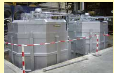
Forced convection pit-type furnaces SAH 5600/75 S in production
