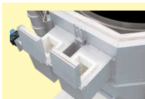
Motor-driven fresh-air and exhaust air flaps
