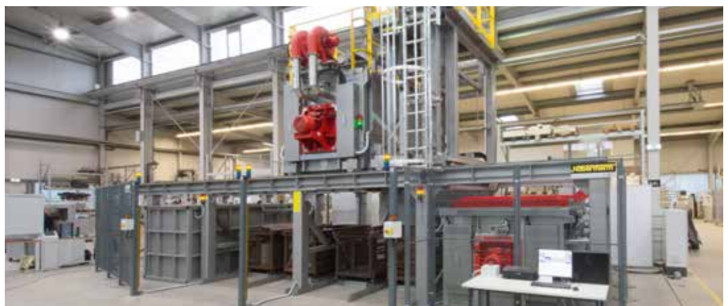
Drop-bottom furnace plant for aluminum
