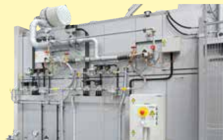
Burner system of gas-fired forced convection bogie hearth furnace WB 4000/85 AS
