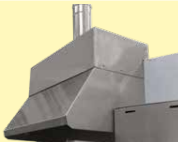
Exhaust hood above charging opening
