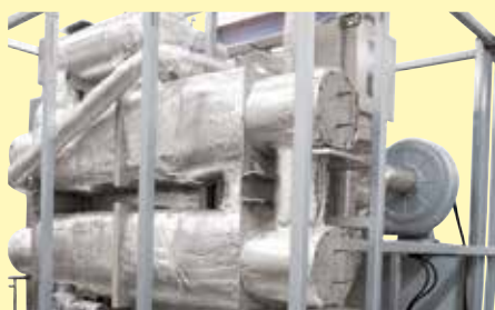
Counterflow heat exchanger for the forced convection chamber furnace N 2560/26 ACLS
