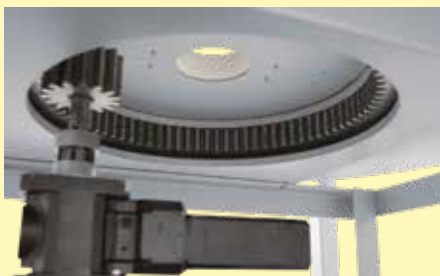
Gear rim drive under the rotary hearth furnace
