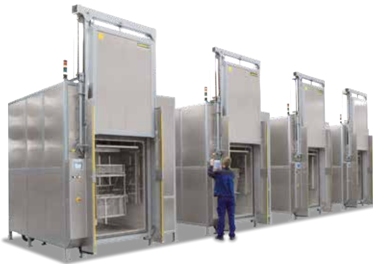
Production system, consisting of four chamber furnaces for moving the load during heat treatment along with a three-stage heat exchanger to optimize energy efficiency
