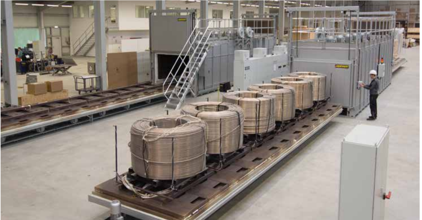
Forced convection bogie hearth furnace W 24750/60AS for annealing aluminum coils
