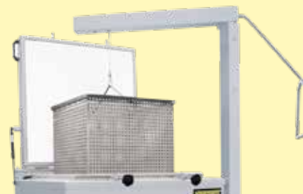
Pit-type furnace SAL 250/85 with charging hoist with swivel arm and charge basket
