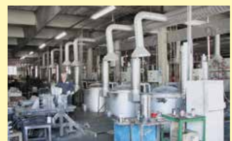
Recuperator burner for aluminum melting furnaces 16 x TBR 110/12 and 2 x TBR 180/12
