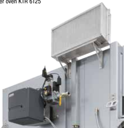
Direct gas-firing at a chamber oven
