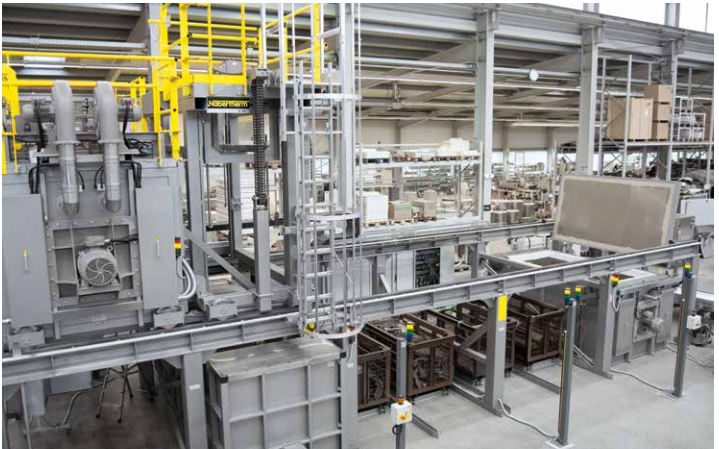
Movable drop-bottom furnace for solution annealing with pit-type furnace for artificial aging with four holding positions
