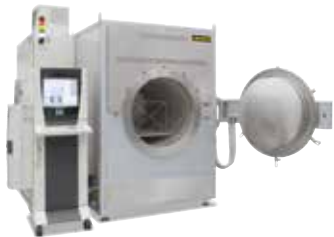
Hot-wall retort furnace NR 300/09 for stress-relief annealing of metal components in protective gas or vacuum after 3D printing
