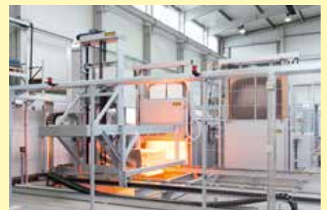
Fully automatic tempering plant for steel
