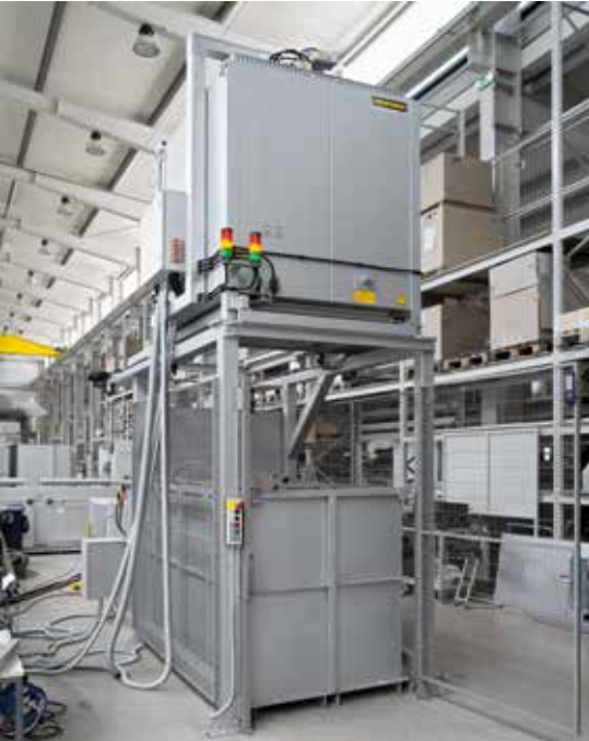
Drop-bottom furnace plant with fixed quench tank (variant A)
