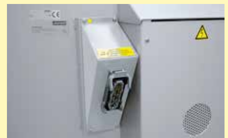
Plug socket on the furnace for the cable connection to the switchgear and control box
