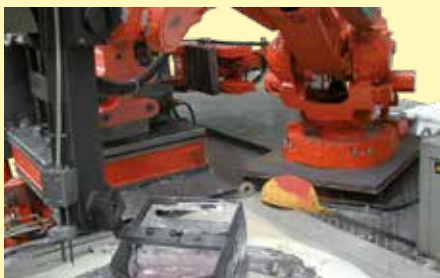
Bale-out of bale-out furnace with robot
