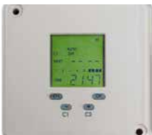
Weekly timer to switch between melting temperature and lower temperature
