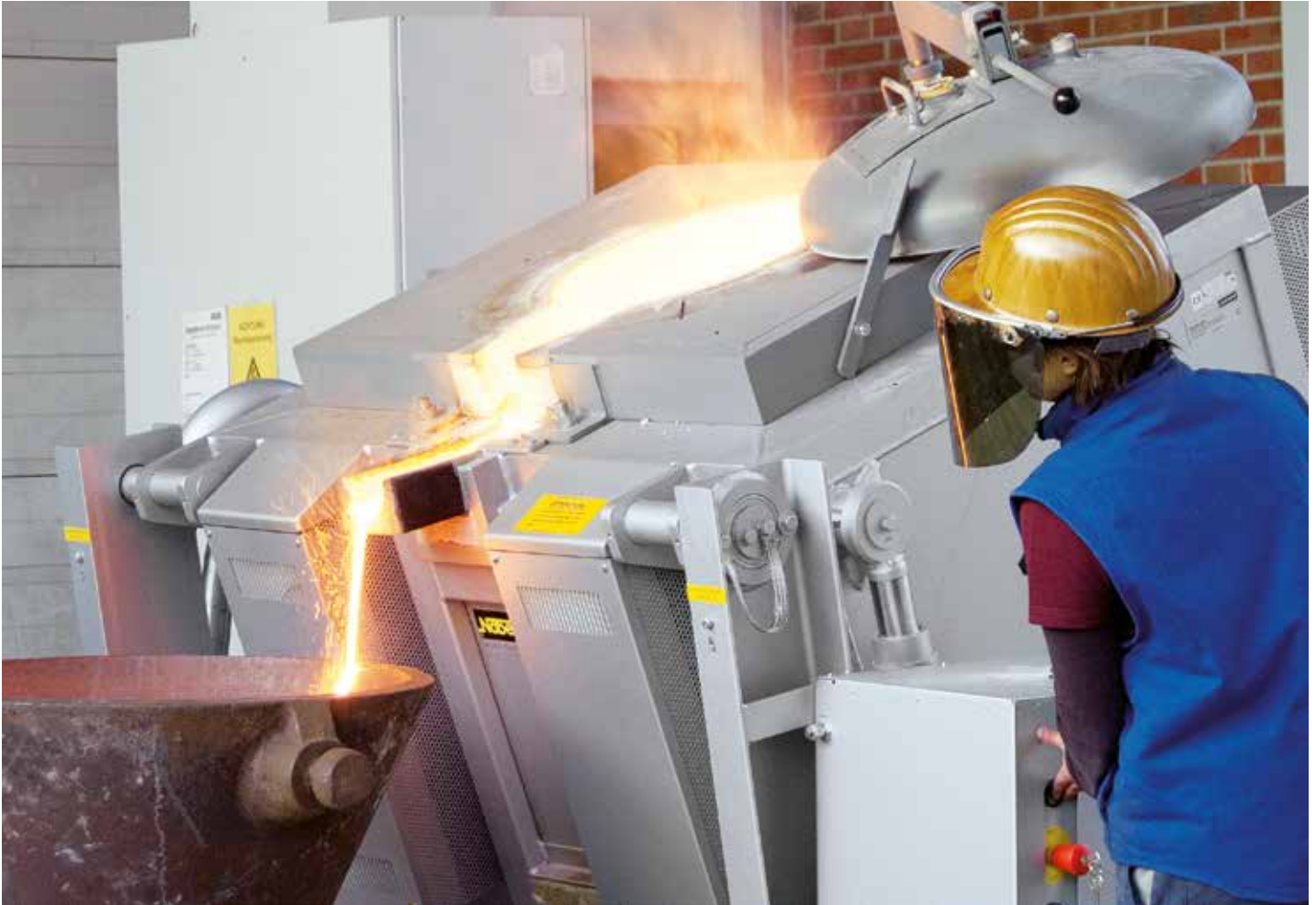
Tilting furnace KC 80/14 during casting
