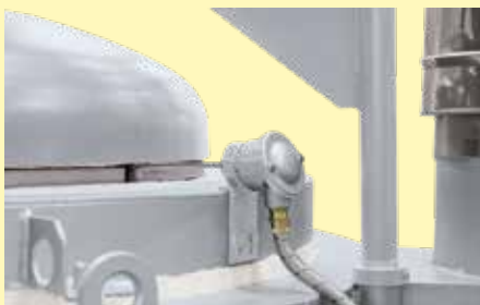
Thermocouple for melt bath control
