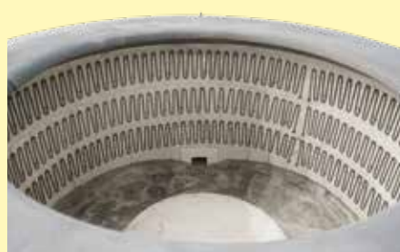
Meander heating elements
