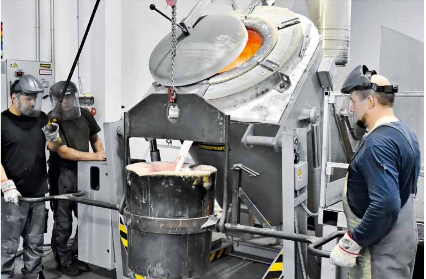
Tilting furnace KB 150/12 in production
