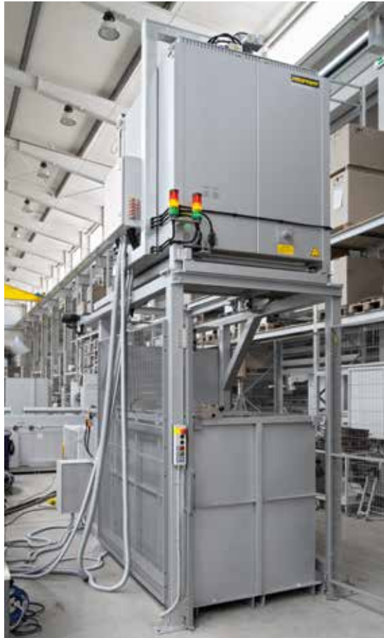
Drop-bottom furnace with fixed quenching bath
