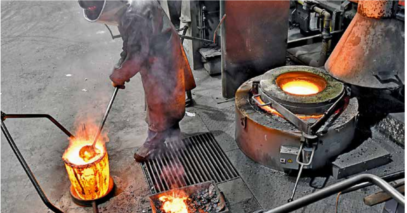
Bale-out furnace TB 20/14 in a pit with exhaust gas discharge over the crucible rime and swiveling collar plate for crucible pulling
