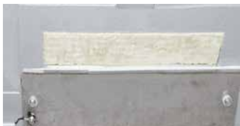
Crucible breakage alarm device under the emergency outlet of a melting furnace
