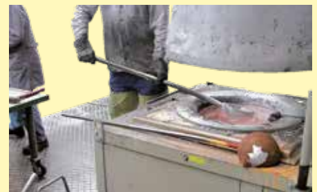
Manual ladling from a bale-out furnace T 80/10
