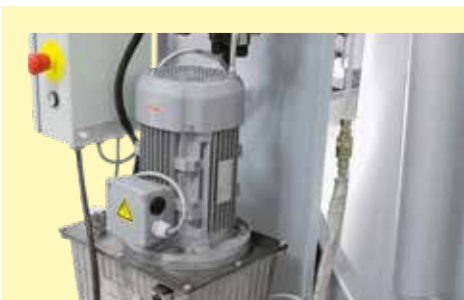
Hydraulic system with flame resistant hydraulic fluid
