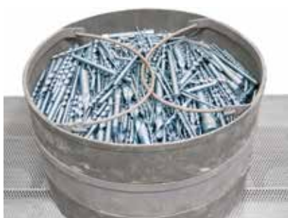
Blueing of drills in water steam atmosphere in a furnace of the NRA range see page 16
