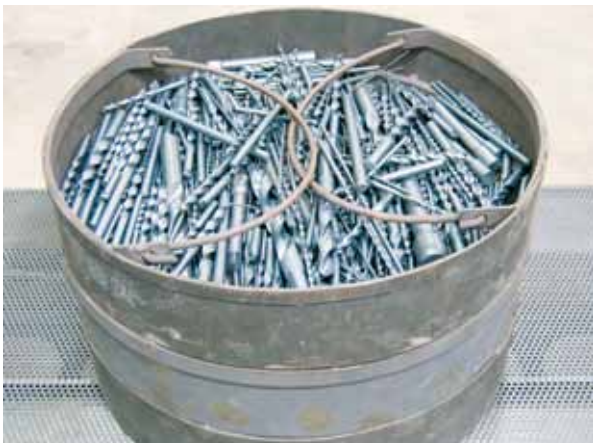
Blueing of drills in water steam atmosphere in a furnace of the NRA range see page 12
